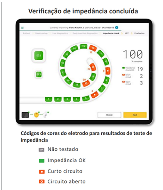
Figure 8: Impedance verification finished with the representation of the situation of the electrodes individually. 12
